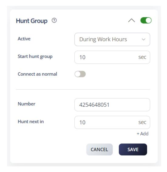
**Time Out:** Each number can have its own timeout before moving on to the next number. The default is 10 seconds timeout for each number.
